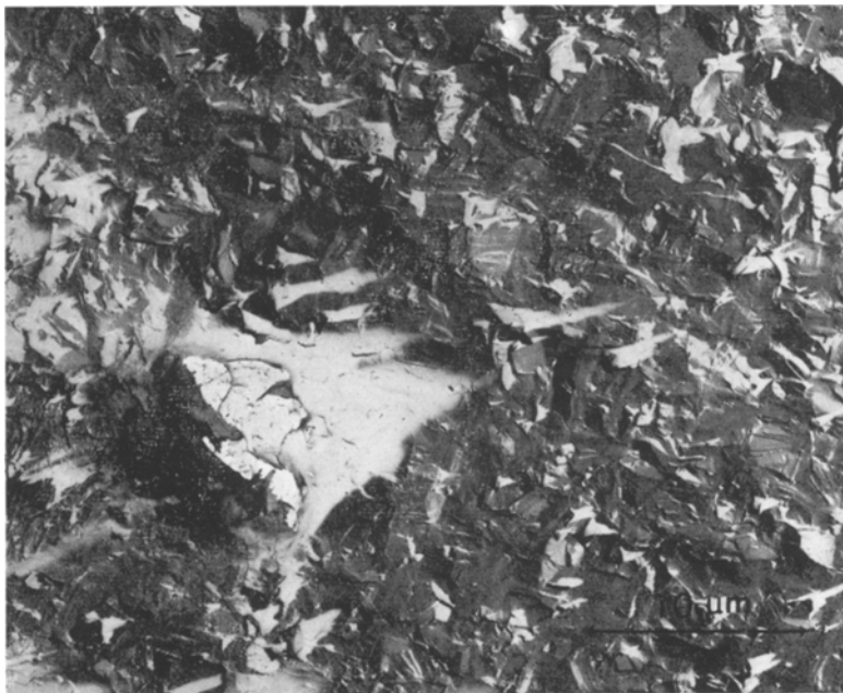
Figure 4 Large particle occurring on the fracture surface of a \beta -alumina test specimen.
